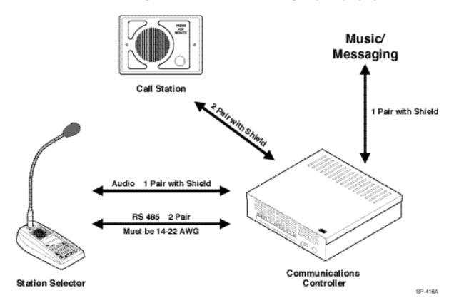
Figure 5. Cable and Connection Requirements
